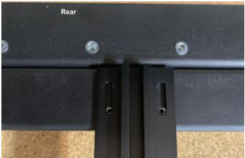
Instal 6 M5x16 SHCS through each t-slot track into the crossmembers and tighten using your torque wrench w/ 4mm hex bit set to 4.5N\*M.
