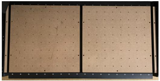
**Note:** Be sure to tighten the screws so they are countersunk from the top of the MDF. This will ensure they are snugly mounted to the X-Carve Pro and allow for the MDF to be planed.
