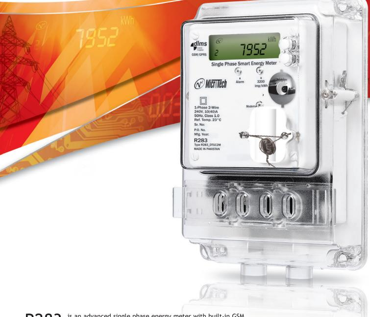
R283 is an advanced single phase energy meter with built-in GSM / GPRS communication module. It is a unique product that comes with DLMS/COSEM certification enabling it to be an ideal candidate for a multi-vendor environment. To resolve energy theft prevalent in local market, R283 is carefully designed with stringent anti-tampering features. To offer highest level of flexibility, it can operate as a standalone product or be integrated with various data collection and energy management tools.
