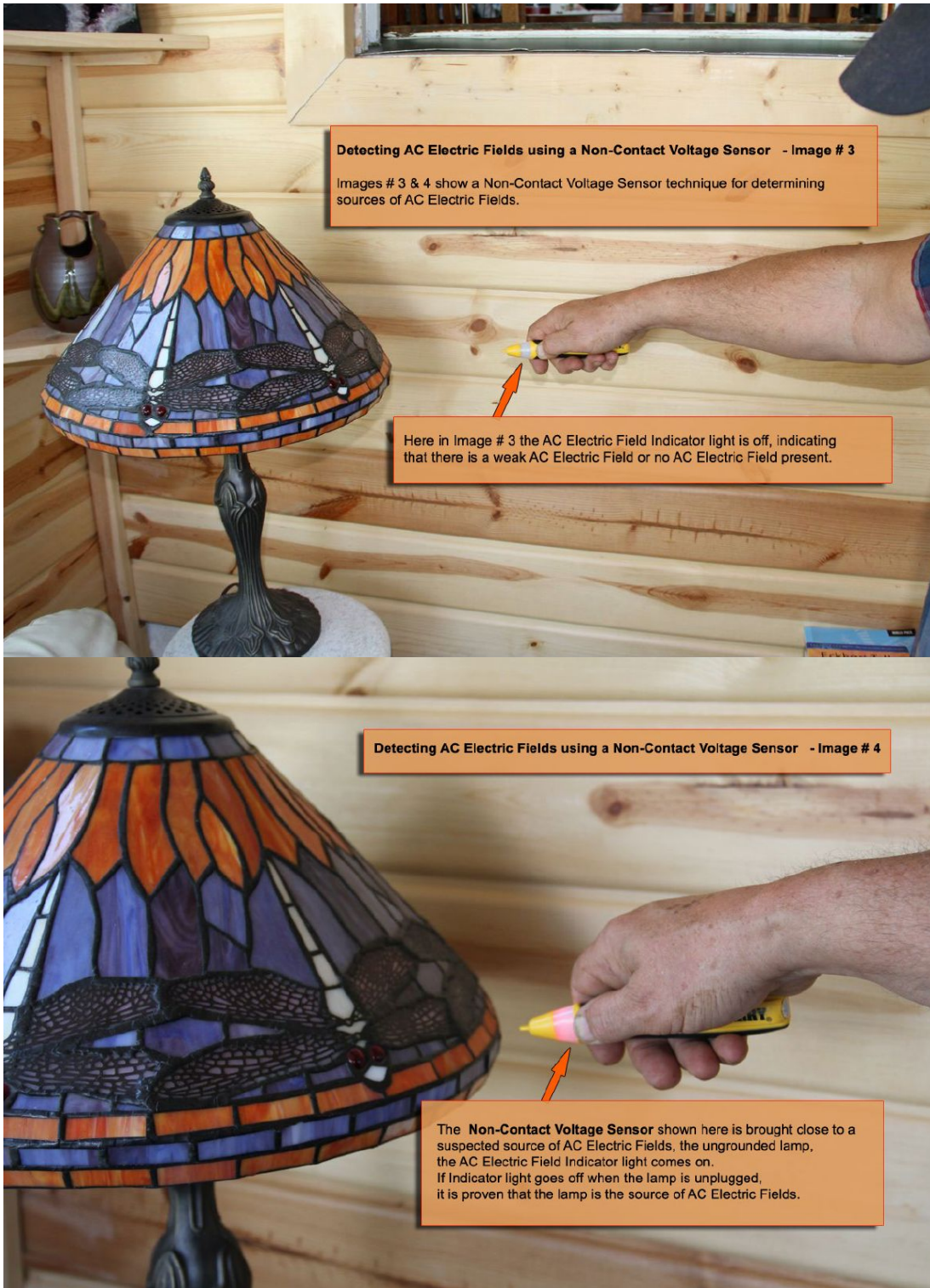
Figure 9: Method of measuring EMFs emitted by appliances using a non-contact voltage sensor. Image #3: the sensor is one foot away from an ungrounded lamp and the indicator light is off, indicating a low level of EMFs. Image #4: the sensor is close to the lamp and the indicator light is on, indicating a high level of EMFs.
