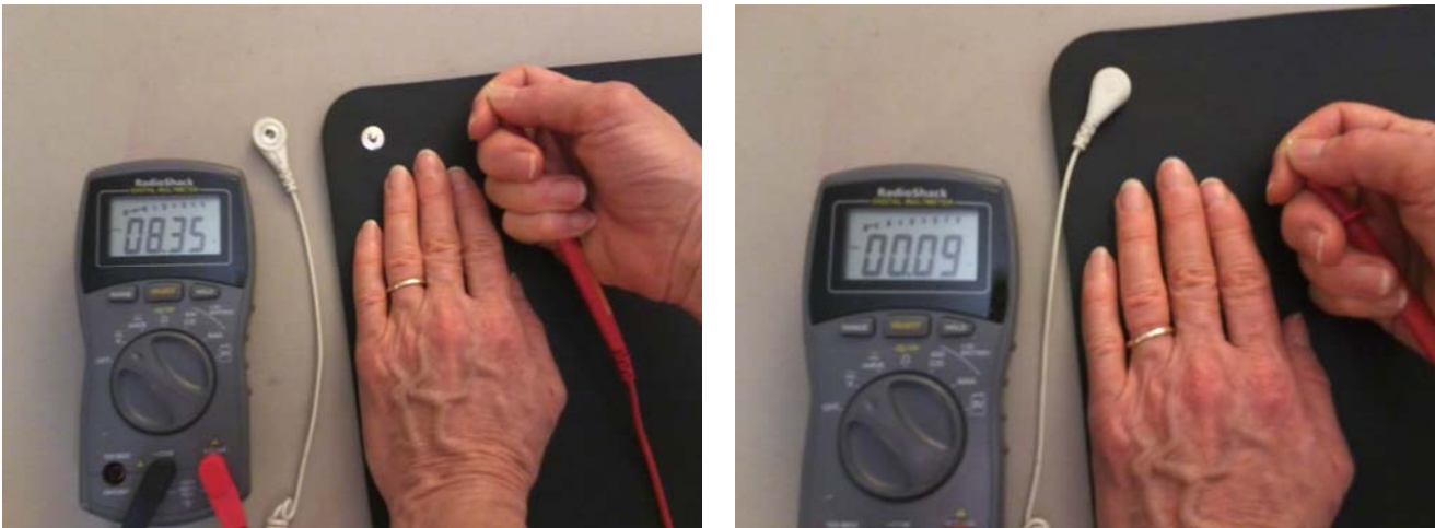
Figure 6: Left: The white grounding wire to the left of the hand is connected to a rod in the ground but it is not touching the grounding mat. The mat and the person touching it are ungrounded. The meter shows a voltage of 8.35 volts induced on the body. Right: The wire is now connected to the grounding mat. The mat is grounded, and when the person touches the mat, she too becomes grounded. The body voltage has dropped to 0.09 volts (90 mV), the level of the EMF background noise.
