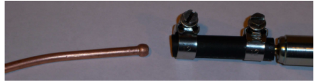
Flared end of copper pipe
