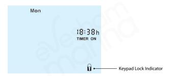
The keypad lock indicator is only visible when the lock is active.
