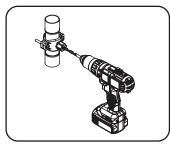
3. For the standard faucets drill a 1/4" hole through one side of the pipe. The drill should be kept straight and centered to avoid damaging the saddle valve. Do not drill through both sides of the pipe!
