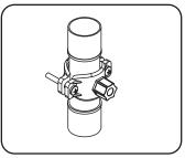
2. Tighten the clamps with the help of the two bolts.
