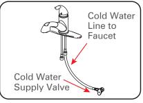
1. Shut off water at supply valve.
