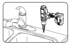
3. Drill a 7/8" hole in the sink using a stepped 7/8" drill bit. If no stepped bit is available, start by drilling a 1/4" hole. Using this hole as a starting point, progressively drill larger holes. Increase drill size by 1/8" until you reach a 7/8" hole.
