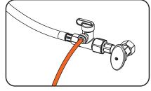
6. Open the cold water supply valve and check for leaks.
