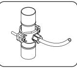
4. Attach 1/4" black tube by slipping the tube through the black compression nut and hand tighten the nut on to the saddle valve.
