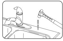
2. Center punch hole to provide a starting point for vour drill.
