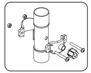
1. Install the drain saddle valve on to the drain pipe. Use 1/4" saddle for drain water line.
