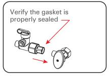
3. Install adapter valve on supply valve.
