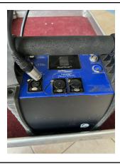
6. Plug the 3-pin XLR into the 24v XLR on your block battery. Make sure if there's a power switch that it's turned on.
