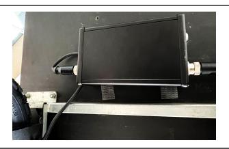
3. You can mount the control box in the desired position with either Dual Lock heavy duty velcro strips, or by drilling two 1/4-inch sized holes in the cart with the supplied **Control Box Drilling Template**.
