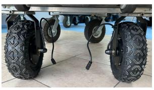
1. Remove the non-Swivel wheel(s) from the cart, and attach motorized wheel(s) with the cable facing inward towards the center of the cart.
