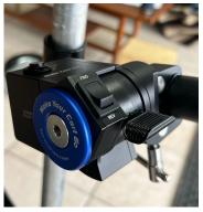
The throttle position can be rotated by loosening the end cap with 7/32 Allen and spinning the clamp on the interior rosettes.
