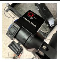
7. Press the Power Switch on the Throttle. The power button will light up & your kit is powered on.
