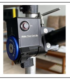
5. Clamp the throttle to your cart in a place where you can steer the cart and still reach the throttle lever.
