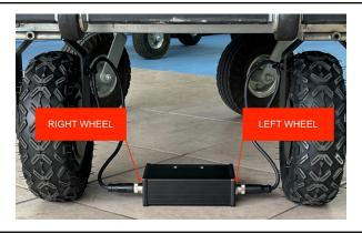
2. Connect wheel cable(s)to the control box.
