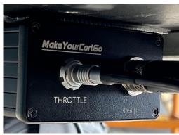
4. Connect Throttle cable to the control box, aligning the red dot with the red indicator.
