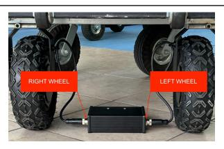
2. Connect wheel cable(s)to the control box.
