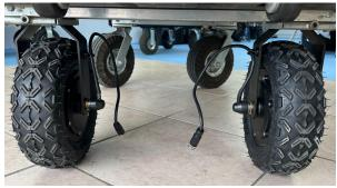
1. Remove the non-Swivel wheel(s) from the cart, and attach motorized wheel(s) with the cable facing inward towards the center of the cart.
