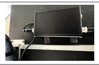
3. You can mount the control box in the desired position with either Dual Lock heavy duty velcro strips, or by drilling two 1/4-inch sized holes in the cart with the supplied **Control Box Drilling Template**.
