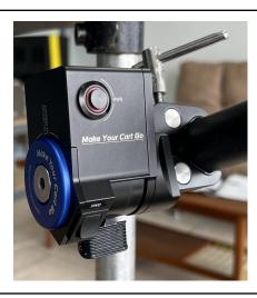
5. Clamp the throttle to your cart in a place where you can steer the cart and still reach the throttle lever.
