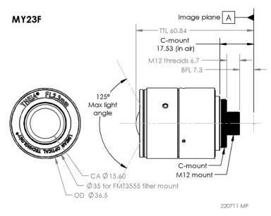
Note: SY23F has both CS-mount and M12 mount threads, however M12 mount threads are partially "internal". For applications requiring M12 mount, order the MY23F version.
