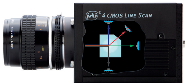
Advanced prism technology supports up to four separate sensors for precise R-G-B values and NIR imaging capabilities. The incoming light is split into 3 or 4 spectral bands (R, G, B) or (R, G, B + NIR) with perfect pixel-to-pixel alignment.
