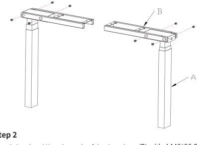
Attach Legs(A) to the Crossbars(B) with 8 M6\*13 Screws (G)
