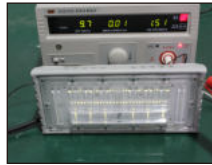
Withstand Voltage Test
