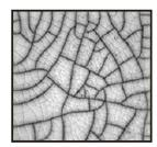
may appear as imperfections, crazing does not affect the performance of life span of your ceramic BBQ; therefore it can't be claimed as a warranty issue. The process of crazing effectively increased the toughness of the unit.
