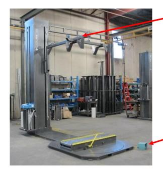
The top fixture mounted on the platen/hold down device is designed to secure the top of the product no matter the shape or size during the wrap cycle.
