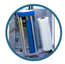
Safety bumpers replace standard safety hoops that are problematic in detecting barriers above floor level and are easily damaged.
