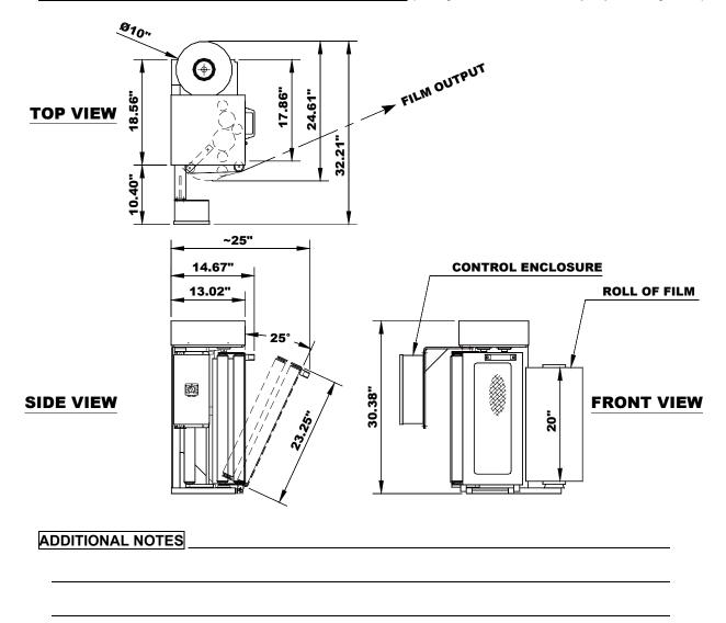
**PLEASE NOTE:** *Rapid Thread* <sup>™</sup> Film Delivery System pre-wired "retro-fit" dispensers are furnished complete (self-contained controls mounted on retro-fit carriage), ready to install and run. The Customer / Distributor is responsible for any mounting bracket attachment, mounting hardware, connecting 115VAC power line from control panel to dispenser and mounting & reconnecting the Auto Load Height Sensing photo-eye (if existing).
