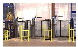
This photo shows three (3) Cousins A-Arm platform automatics installed in a strategic location at a major beverage distribution center. The layout allows the operator to place a pallet on a machine that is empty and then pick a wrapped pallet from another machine. They are installed in pits so they can be used with all types of material handling equipment.
