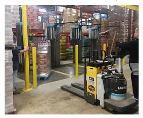
Photo shows (3) Cousins LP-SWA installed in pits at a major beer distribution center. The pit installation allows the machines to be used with all types of material handling equipment.
