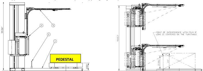
Another solution is to modify the turntable/base moving the turntable closer to the machine tower which positions the load closer to the film web. This option is a factory quote.
