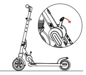
2. Then step down the folding lever to put down the stem.
