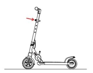
4. Tighten the stem lock with a 5mm Allen wrench.
