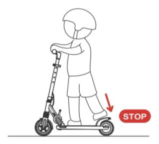
3. Step on the rear fender brake with your foot.
