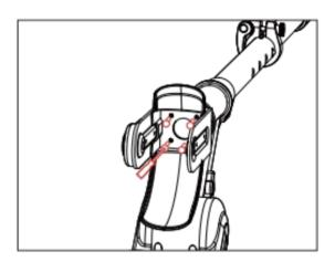
2.2. Insert the two spacers into the wheel hub. Put the front wheel between the dropouts of the front fork. Pass the wheel axle through either dropout and the wheel hub. Pass the big cross-head screw through the other dropout and spin it into the axle. Then tighten the screw with the included screwdriver.
