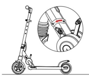
1. First, confirm that the electric scooter has been turned off. Hold the handlebar with one hand and spin the safety switch to unlock position.
