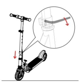
3. After removing the electric scooter, assemble the stem to the -e-scooter body.
