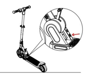
1. Press the power switch to turn on the e-scooter, and there will be a prompt sound. (Tips: Please wear protective equipment such as a helmet, kneepads, and elbow pads before riding.)
