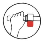
2. Press and hold the red thumb brake to realize fast braking;
