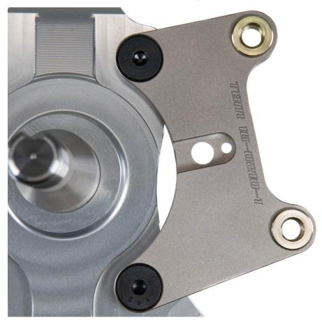
**Step 5:** Install wheel and rotor assembly onto the spindle, pack outer bearing and install in wheel. Secure assembly with the flat washer and spindle castle nut.
