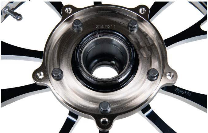
Step 2: Lay the wheel face down and place the flat side of rotor on the hat.
