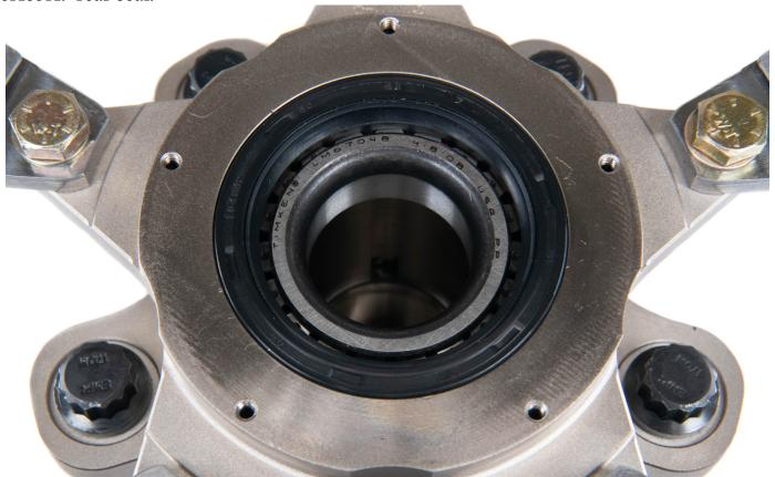
**Step 6**. Mount the caliper bracket using the 3/8-16 bolts, then torque to factory spec. If purchased, install your wheel speed sensor.
