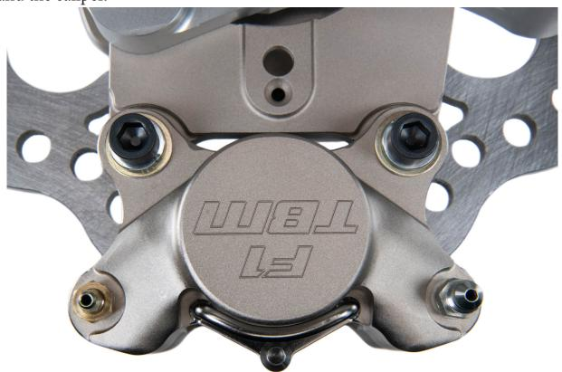
**Step 9:** Remove the pad retainer bolt (if already inserted). Insert the brake pads from the top of the caliper and reinsert the pad retainer bolt. Hold the pads against the caliper housing. Spin the rotor assembly to check for contact between the rotor and brake pads. There should be no contact between the rotor and pads. Be sure to tighten the pad retainer bolt once pads are installed.
