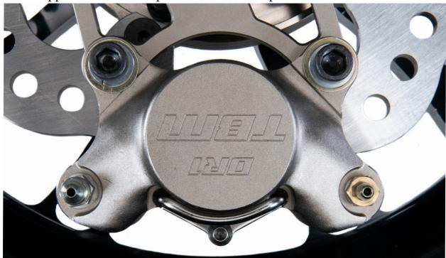
**Step 7:** Remove the pad retainer bolt. Insert the brake pads from the top of the caliper and reinsert the pad retainer bolt. Hold the pads against the caliper housing. Spin the rotor assembly to check for contact between the rotor / pads. There should be no contact between the rotor / pads. If the pads contact the rotor caliper shimming with supplied shims (.010, .031 .062) may be required. Be sure to tighten the pad retainer bolt.
