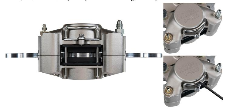
**Step 8:** If there is pad to rotor contact, determine which side is causing the interference. Shim the caliper or the bracket as needed using the supplied shim kit to center the caliper and ensure the caliper is parallel to the rotor. \*\*What is required for one side of the car may not be the same as the other side. Check each side individually\*\*
