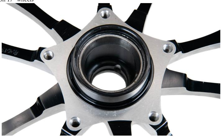
**Step 5:** Pack inner bearing with grease and insert into back side of wheel, install Strange style seal (Timken 40494S or National 473454) supplied with your wheels.
