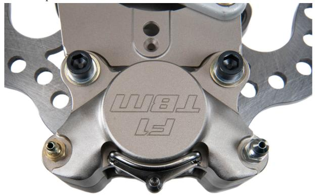
**Step 9:** Remove the pad retainer bolt (if already inserted). Insert the brake pads from the top of the caliper and reinsert the pad retainer bolt. Hold the pads against the caliper housing. Spin the rotor assembly to check for contact between the rotor and brake pads. There should be no contact between the rotor and pads. Be sure to tighten the pad retainer bolt once pads are installed.
