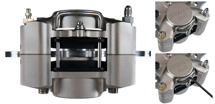
**Step 10:** If there is pad to rotor contact, determine which side is causing the interference. Shim the caliper or the bracket as needed using the supplied shim kit to center the caliper and ensure the caliper is parallel to the rotor. \*\*What is required for one side of the car may not be the same as the other side. Check each side individually\*\*
