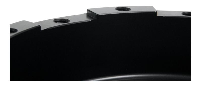
**Step 4**: Place the Rotor with the flat side down on the taller step of the Rotor Hat, apply Red Loctite to the 5/16 -18 hex bolts, torque to 18 ft-lbs.
