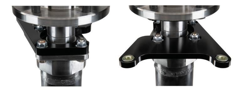
**Step 3:** When mounting the rotor on the hat, each hat has 2 steps and each rotor can be mounted two ways to accommodate different axle offsets and machining tolerances. This allows you to configure the perfect rotor position depending on your vehicle.
