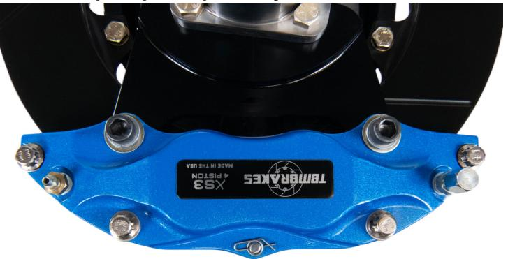
**Step 7:** Spin the axle assembly to ensure the rotor spins free of any contact with the rotor bolts and the caliper bracket. The complete assembly should look like the photo below.
