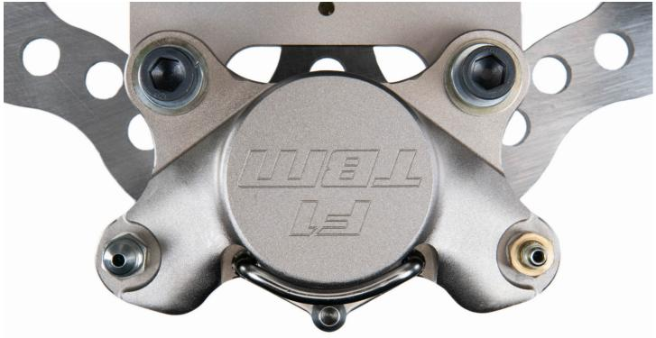
**Step 7:** Remove the pad retainer bolt (if already inserted). Insert the brake pads from the top of the caliper and reinsert the pad retainer bolt. Hold the pads against the caliper housing. Spin the rotor assembly to check for contact between the rotor and brake pads. There should be no contact between the rotor and pads. Be sure to tighten the pad retainer bolt once pads are installed.
