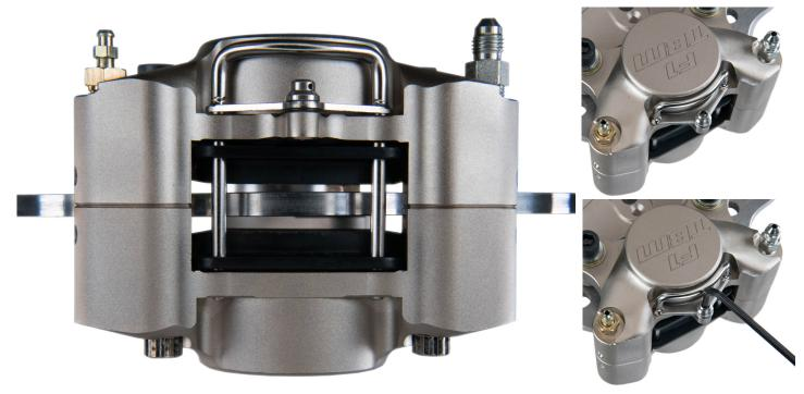
**Step 8:** If there is pad to rotor contact, determine which side is causing the interference. Shim the caliper or the bracket as needed using the supplied shim kit to center the caliper and ensure the caliper is parallel to the rotor. \*\*What is required for one side of the car may not be the same as the other side. Check each side individually\*\*
