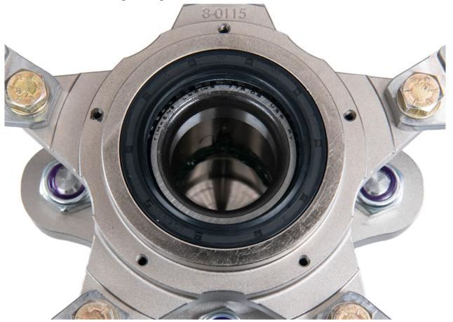
**Step 4**: Mount the caliper bracket using the 3/8-16 FHCS bolts and then torque to 37 ft-lbs.
