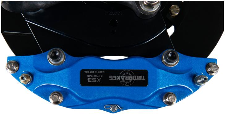
**Step 10:** Remove the pad retainer pin (if already inserted). Insert the brake pads from the top of the caliper and reinsert the pad retainer pin. Hold the pads against the caliper housing. Spin the rotor assembly to check for contact between the rotor and brake pads. There should be no contact between the rotor and pads. Be sure to reinstalled the pad retainer pin and clip once pads are installed.
