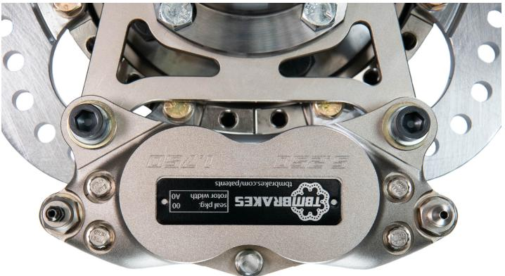
**Step 7:** Spin the axle assembly to ensure the rotor spins free of any contact with the rotor bolts and the caliper bracket. The complete assembly should look like the image below.
