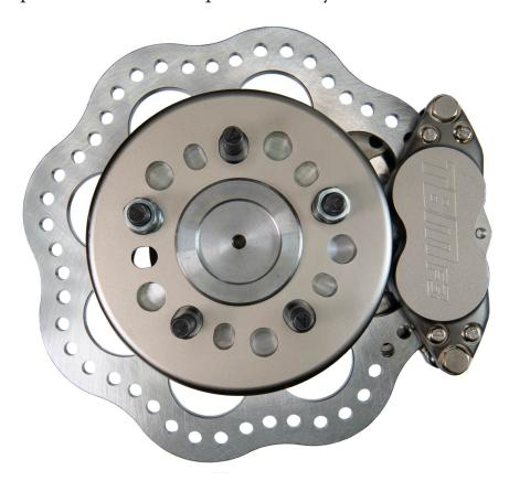
**Step 8:** Remove the pad retainer pin and clip (if already inserted). Insert the brake pads from the top of the caliper and reinsert the pad retainer pin. Hold the pads against the caliper housing. Spin the rotor assembly to check for contact between the rotor and brake pads. There should be no contact between the rotor and pads. Be sure to reinstall the pin and clip once pads are installed.
