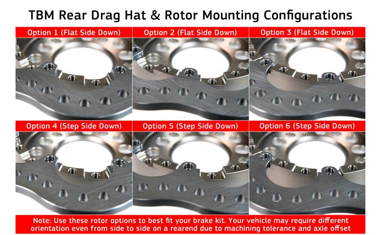
**Step 4**: Once the correct rotor height has been achieved apply Red Loctite to the eight 5/16-18 hex bolts, torque to 18 ft-lbs.
