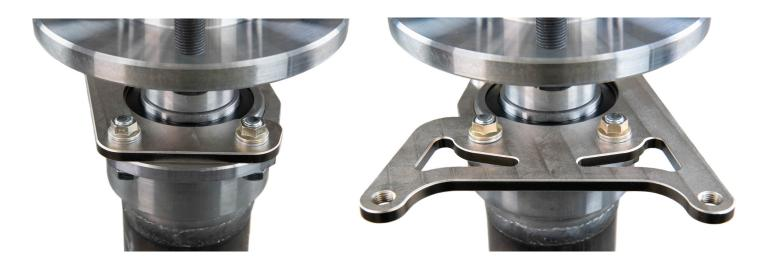
**Step 3:** When mounting the rotor on the hat, each hat has 3 steps and each rotor is stepped to accommodate different axle offsets and machining tolerances. This allows you to configure the perfect rotor position depending on your vehicle.
