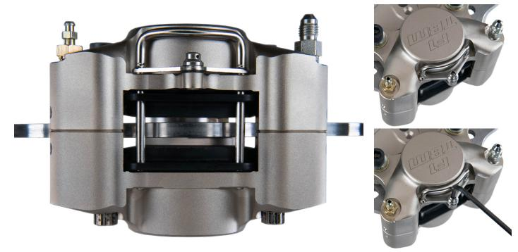
**Step 10:** If there is pad to rotor contact, determine which side is causing the interference. Shim the caliper or the bracket as needed using the supplied shim kit to center the caliper and ensure the caliper is parallel to the rotor. \*\*What is required for one side of the car may not be the same as the other side. Check each side individually\*\*
