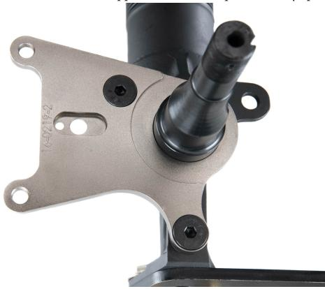
**Step 7.** Pack outer bearing and install in wheel. Install wheel and rotor assembly onto the spindle and secure with the washer and castle nut.
