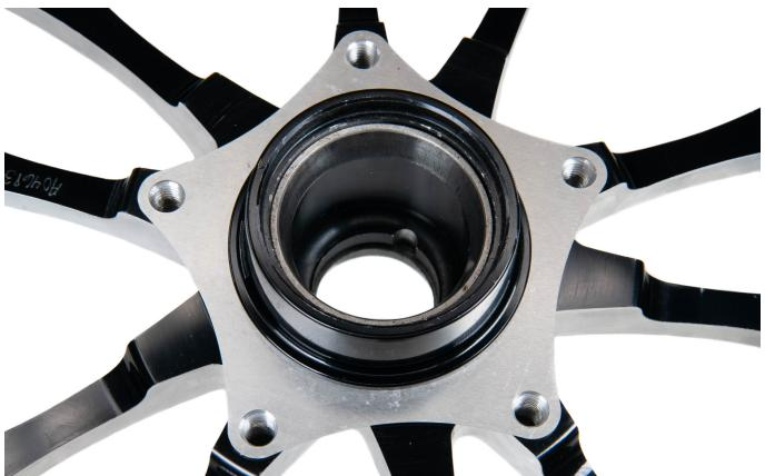
**Step 3:** Lay the wheel face down and place the flat side of rotor on the hat.
