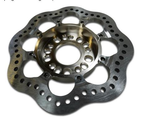
**3.** Apply red Loctite to the 5/16-18 hex bolts, torque to 18 ft-lbs. (Important: do not Loctite or torque bolts until proper fitment is achieved)
