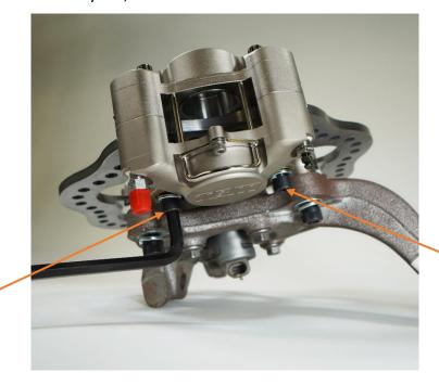
**7.** Remove the pad retainer (if already inserted). Insert the brake pads, reinsert the pad retainer, and hold the pads against the caliper housing. Spin the rotor assembly to check for contact between the rotor and brake pads. There should be no contact between the rotor and pads.
