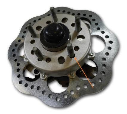
**6.** Slide the caliper over the rotor and mount it to the bracket. Snug the 3/8-24 bolts, lock washer and washer, torque to 37 ft-lbs. Check for proper radial and horizontal clearance between the rotor and the caliper. If needed, loosen the 7/16-14 bolts and pull up on the caliper to get adequate rotor to caliper clearance. (.050"). Also check to make sure the bolts are not touching the rotor. If they are, add shims.
