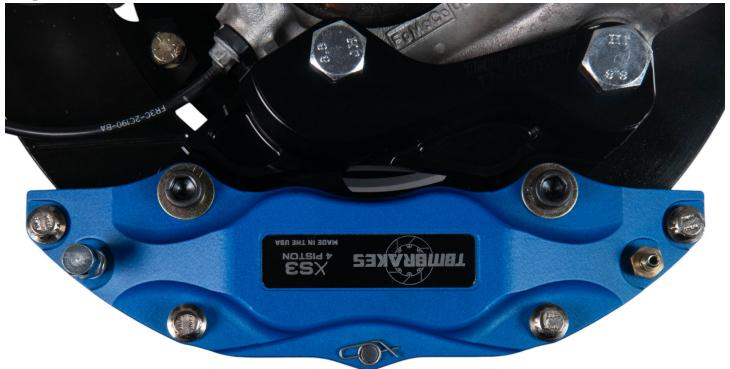
**Step 8:** Remove the pad retainer pin (if already inserted). Insert the brake pads from the top of the caliper and reinsert the pad retainer pin. Hold the pads against the caliper housing. Spin the rotor assembly to check for contact between the rotor and brake pads. There should be no contact between the rotor and pads. Be sure to reinstalled the pad retainer pin and clip once pads are installed.
