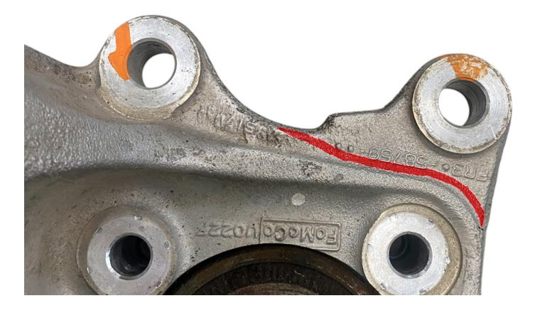
**Step 3:** Once the mounting ear of the knucle has been trimmed off, your knuckle should
