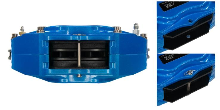
**Step 9:** If there is pad to rotor contact, determine which side is causing the interference. Shim the caliper or the bracket as needed using the supplied shim kit to center the caliper and ensure the caliper is parallel to the rotor. \*\*What is required for one side of the car may not be the same as the other side. Check each side individually\*\*
