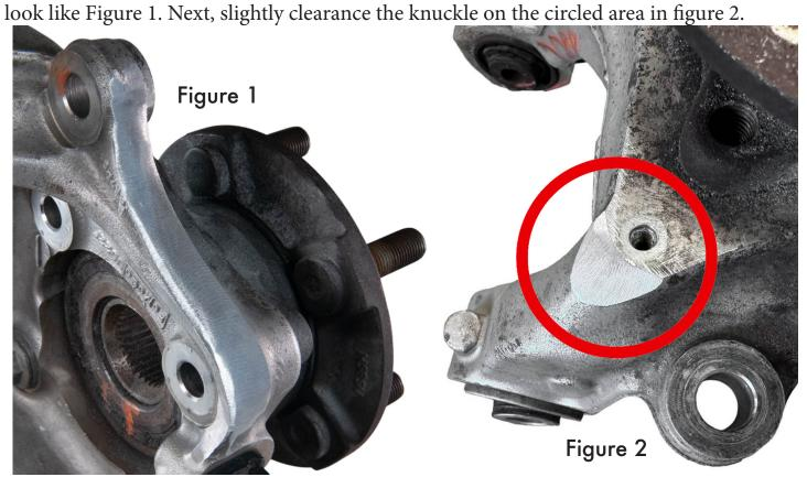
**Step 4:** Remove the lower factory hub bolt (not pictured) closest to the trimmed ear and bolt on the caliper bracket using the M12 X1.50 hex bolt. Then place the M14 hex bolt in
