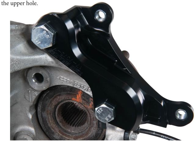
**Step 5:** Use the M14 locknut on the front side of the knuckle and tighten to 80ft/lbs. Now you can torque the lower M12 bolt to 60ft/lbs.
