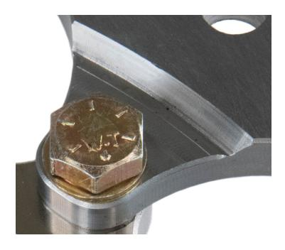
**Step 3:** Place the caliper bracket over the factory caliper ears and install using the supplied M14 hardware.
