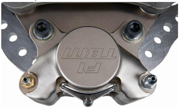
**Step 6:** Remove the pad retainer bolt (if already inserted). Insert the brake pads from the top of the caliper and reinsert the pad retainer bolt. Hold the pads against the caliper housing. Spin the rotor assembly to check for contact between the rotor and brake pads. There should be no contact between the rotor and pads. Tighten pad retainer bolt.
