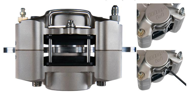
**Step 7:** If there is pad to rotor contact, determine which side is causing the interference. Shim the caliper or the bracket as needed using the supplied shim kit to center the caliper and ensure the caliper is parallel to the rotor. \*\*What is required for one side of the car may not be the same as the other side. Check each side individually\*\*
