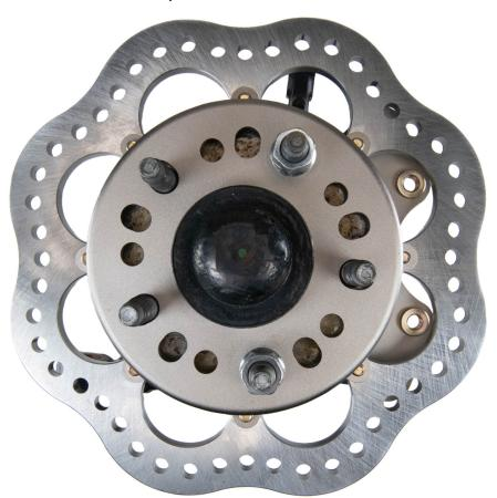
**Step 5:** Slide the caliper over the rotor and mount it to the bracket. Snug the 3/8-24 bolts, lockwasher, and washer. Check for proper radial and horizontal clearance between the rotor and the caliper.
