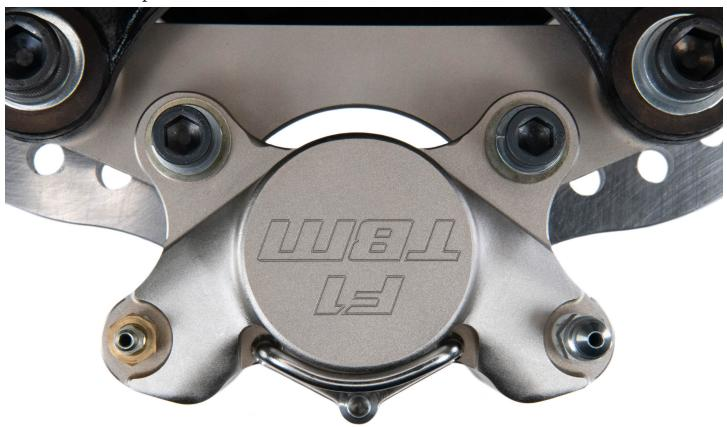
**Step 6:** Remove the pad retainer bolt (if already inserted). Insert the brake pads from the top of the caliper and reinsert the pad retainer bolt. Hold the pads against the caliper housing. Spin the rotor assembly to check for contact between the rotor and brake pads. There should be no contact between the rotor and pads. Tighten pad retainer bolt.
