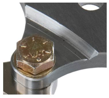
**Step 3**. Place the caliper bracket over the knuckle as shown and use the supplied M12 bolts, lockwasher, and washer to bolt the bracket from the front side of the knuckle. Note: The .250 aluminum spacers are only used with strange hubs.
