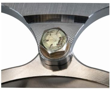
**Step 3**: Place the caliper bracket on the face of the knuckle as shown below. Apply red Loctite to the M8 X 1.25 X 20MM SHCS and tighten to 22ft/lbs.
