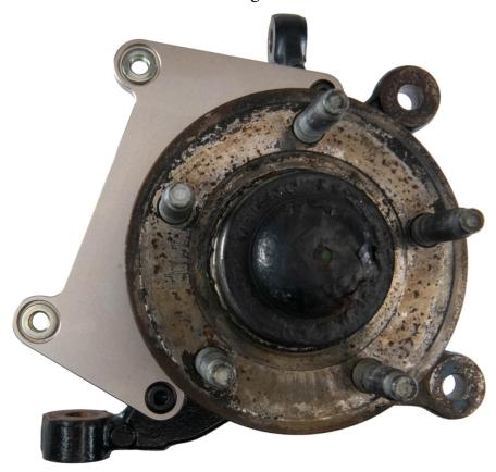
**Step 4:** Slide hat and rotor assembly onto the hub and secure the hat flush to the hub by using two lug nuts.
