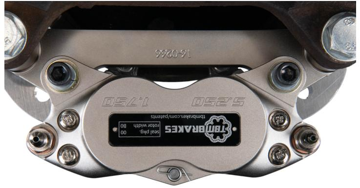
**Step 6:** Remove the pad retainer bolt (if already inserted). Insert the brake pads from the top of the caliper and reinsert the pad retainer bolt. Hold the pads against the caliper housing. Spin the rotor assembly to check for contact between the rotor and brake pads. There should be no contact between the rotor and pads. Be sure to tighten the pad retainer bolt once pads are installed.
