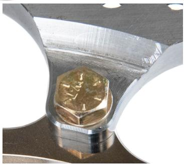
**Step 4.** Mount the bracket to the spindle using the M12 x 1.75 bolt in the upper hole and the  $3/8-24 \times 1.375$  allen bolt, washer, and lock washer in the lower hole; torque to factory
