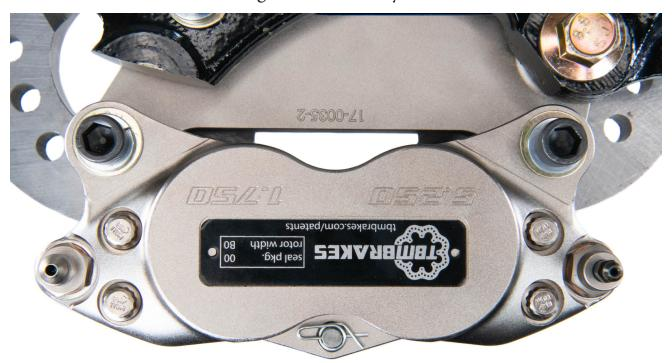
**Step 7:** Remove the pad retainer bolt (if already inserted). Insert the brake pads from the top of the caliper and reinsert the pad retainer bolt. Hold the pads against the caliper housing. Spin the rotor assembly to check for contact between the rotor and brake pads. There should be no contact between the rotor and pads. Tighten pad retainer bolt.
