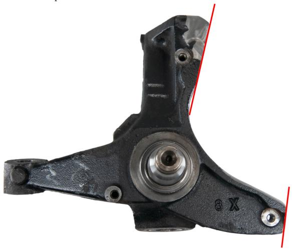
Use a cut off wheel or tool of choice to make your cuts, however be sure to not damage the spindle shaft.
