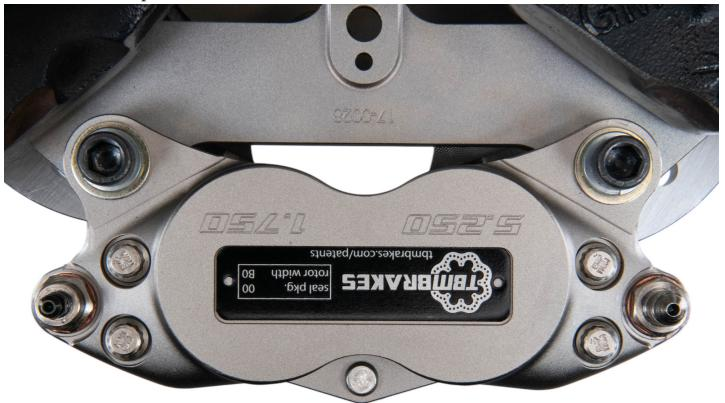
**Step 9:** Remove the pad retainer bolt (if already inserted). Insert the brake pads from the top of the caliper and reinsert the pad retainer bolt. Hold the pads against the caliper housing. Spin the rotor assembly to check for contact between the rotor and brake pads. There should be no contact between the rotor and pads. Be sure to tighten the pad retainer bolt once pads are installed.
