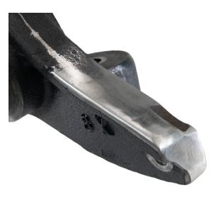
**Step 1:** Remove the existing brake components and ensure the spindle is clean and free of debris.
