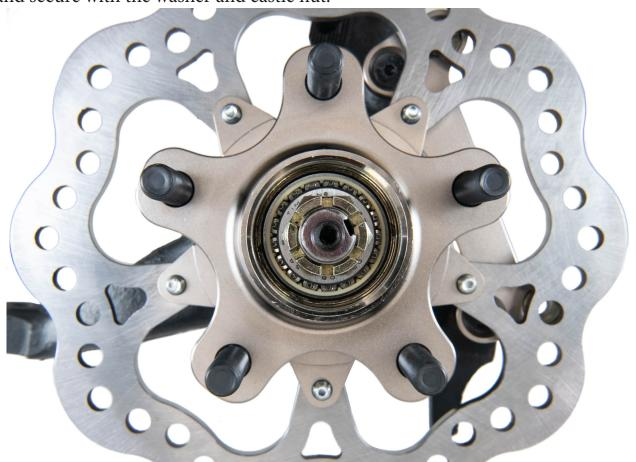
**Step 8:** Slide the caliper over the rotor and mount it to the bracket. Snug the 3/8-24 bolts, lock washer, and washer. Check for proper radial and horizontal clearance between the rotor and the caliper.
