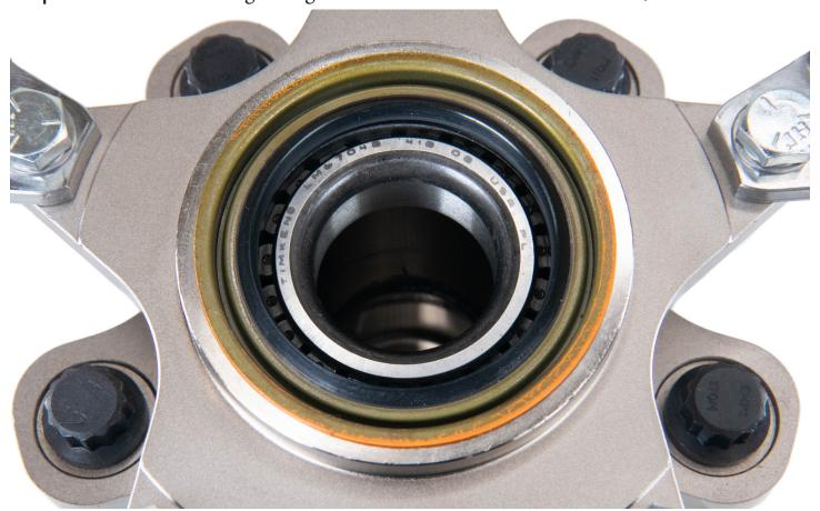
**Step 6.** Mount the caliper bracket using the 3/8-24 allen bolts, then torque to 37ft/lbs.
