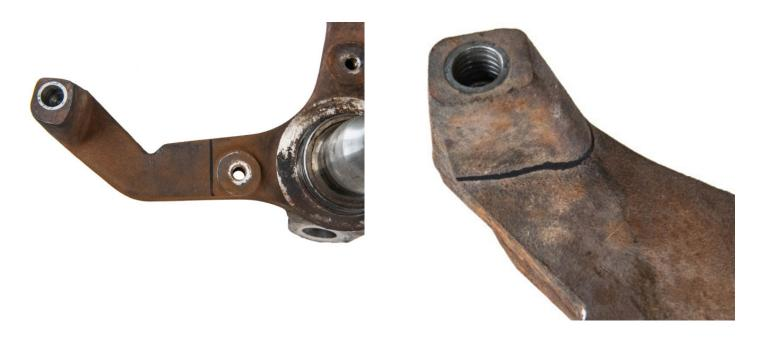
Use a cut off wheel or tool of choice to make your cuts, however be sure to not damage the spindle shaft.
