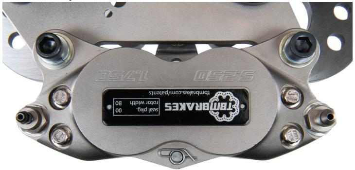
**Step 9:** Remove the pad retainer bolt (if already inserted). Insert the brake pads from the top of the caliper and reinsert the pad retainer bolt. Hold the pads against the caliper housing. Spin the rotor assembly to check for contact between the rotor and brake pads. There should be no contact between the rotor and pads. Be sure to tighten the pad retainer bolt once pads are installed.
