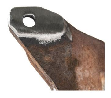
**Step 1:** Remove the existing brake components and ensure the spindle is clean and free of debris.
