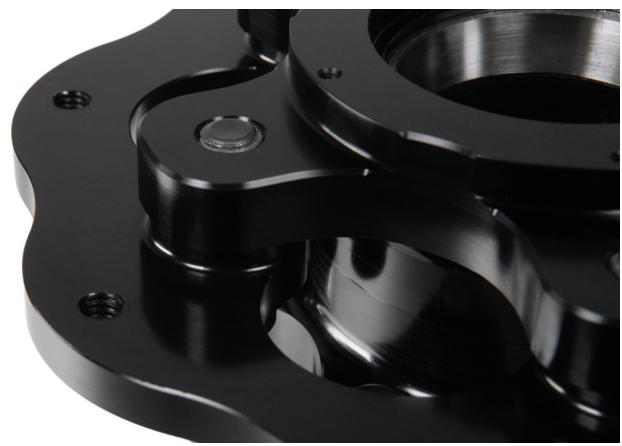
**Step 5:** Place the Rotor with the flat side down on the Rotor Adapter, apply Red Loctite to the 5/16 -18 hex bolts, torque to 18 ft-lbs.
