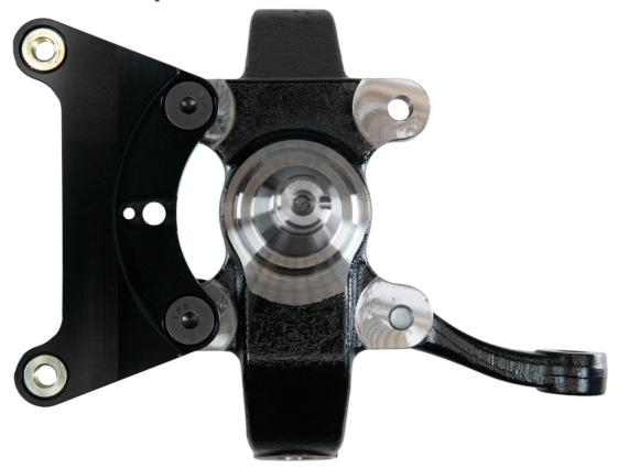
**Step 9:** Place the aluminum spacer between the steering arm and the mounting ear as shown below. Install the 7/16-14 nylon nut on the end of the bolt and torque to 37ft/lbs. Torque the upper 7/16-20 bolt to 37ft/lbs.
