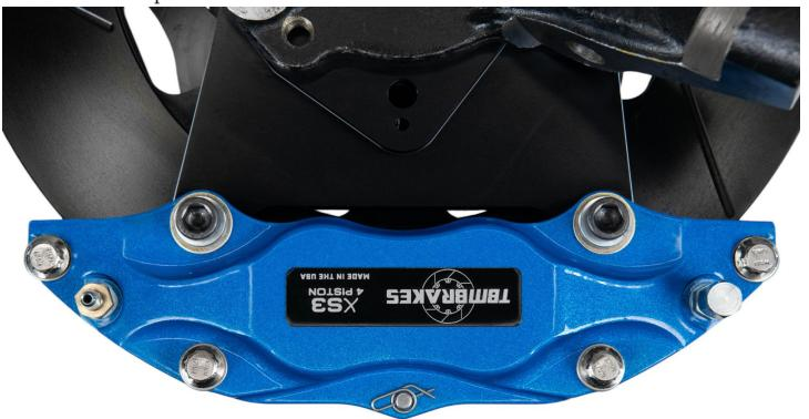
**Step 10:** Remove the pad retainer pin (if already inserted). Insert the brake pads from the top of the caliper and reinsert the pad retainer pin. Hold the pads against the caliper housing. Spin the rotor assembly to check for contact between the rotor and brake pads. There should be no contact between the rotor and pads. Be sure to reinstalled the pad retainer pin and clip once pads are installed.
