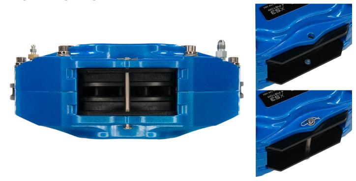
**Step 11:** If there is pad to rotor contact, determine which side is causing the interference. Shim the caliper or the bracket as needed using the supplied shim kit to center the caliper and ensure the caliper is parallel to the rotor. \*\*What is required for one side of the car may not be the same as the other side. Check each side individually\*\*
