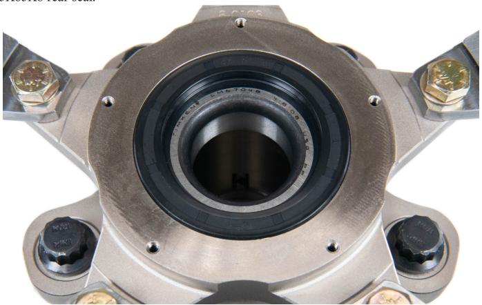
**Step 6:** For disc brake spindles place the aluminum .500" spacer over the top hole and place three .031" shims over the lower mounting hole. Next bolt on the caliper bracket using the 5/8-18 X 1.25" FHCS and torque to 80ft/lbs. Then install the 1/2-13 FHCS, washer, and nylock nut and torque to 60ft/lbs.
