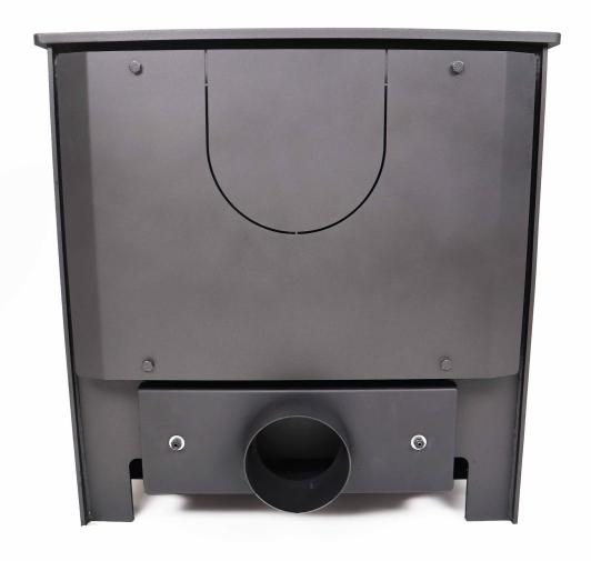
Congratulations, you have successfully installed the direct air adaptor to your Woolly Mammoth mkii stove. Now attach a 4" pipe or hosing to the outlet at the back and seal with fire cement. Pass the pipe through an external wall and your stove will no longer take air from the room.
