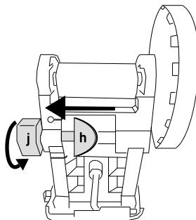
**Dial Manual Resistance Knob (j) clockwise so the flat portion of the Semi-Circular Adjuster (h) is nearest the outer casing of the Resistance Unit.**
