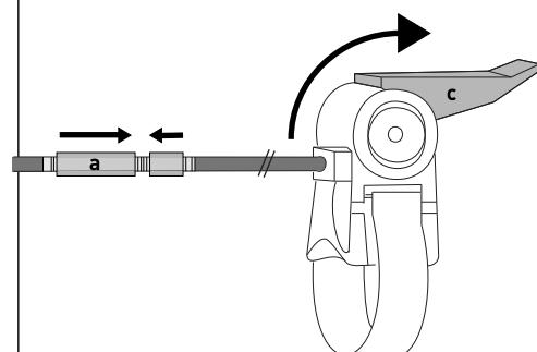
**Tighten and thread the Barrel Adjuster (a) into the closed position. Press the Shifting Lever (c) on the Remote Shifter completely to the DOWN position.**
