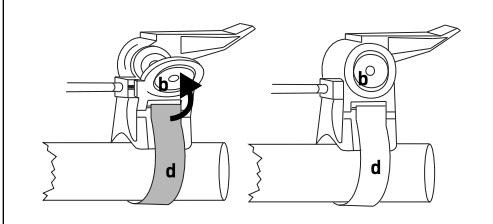
**Adjust the Nylon Strap (d) to fit snugly around the bike's handle bar. Flip the Cam Lock (b) up and into the locked position. If the Cam Lock (b) does not secure the Remote Shifter, make further adjustments to the Nylon Strap (d) and re-engage the Cam Lock (b).**
