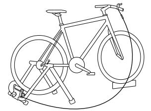
**Route the Remote Shifter Cable around the bike and up to the bike's handle bar.
