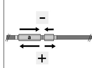
**Loosen or tighten the tension on the shifting cable by threading the Barrel Adjuster (a) in or out.**
