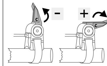
**Adjust the resistance on your trainer using the Remote Shifter. To decrease resistance, lift the Shifting Lever (c) into the upright position. To increase resistance, push the Shifting Lever (c) into the down position.**
