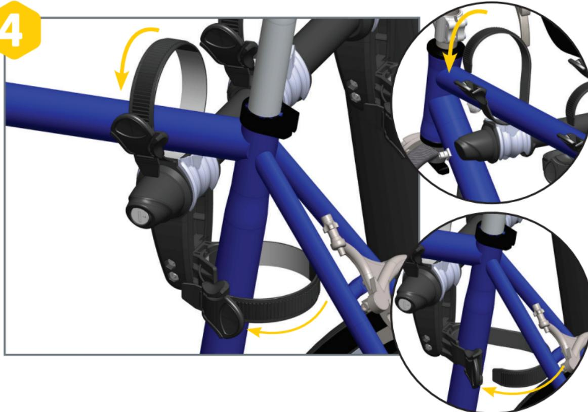
**EN** Insert straps through buckles and pull tightly around bike frame. The top straps secure the top tube of bicycle. The anti-sway straps that hang below the rack arms secure the bike's vertical seat tube.
