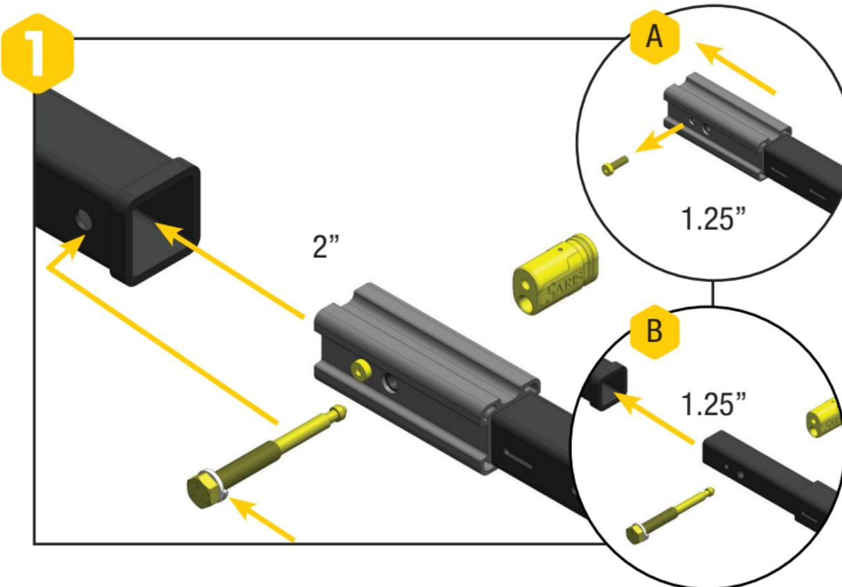
**EN** Install receiver tube into hitch. Install lock washer on hitch pin. Hitch pin should enter in on the driver's side. Tighten hitch pin with wrench. Secure with lock.
