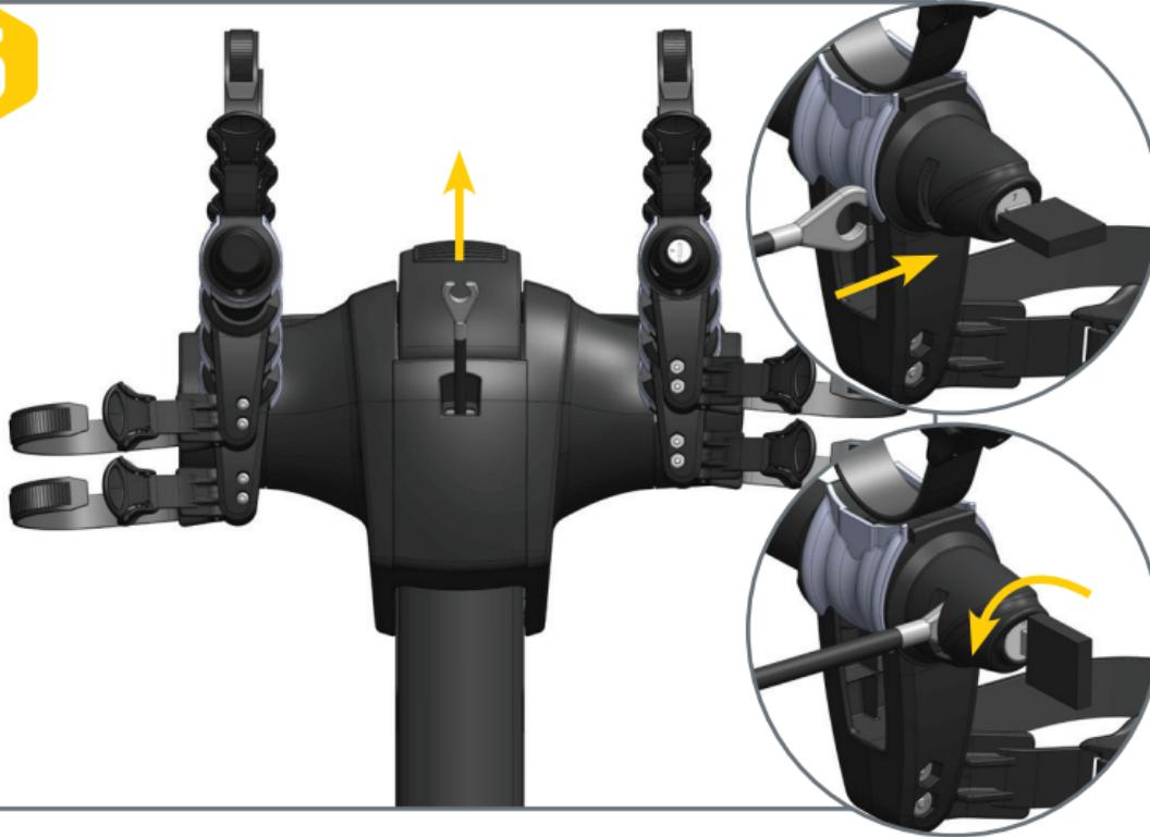
**EN** To lock bikes with integrated lock, pull cable lock out of housing, loop over top of bikes and insert cable into end of right arm. Turn key to lock.
