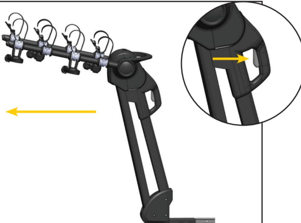
**EN** While standing between the rack and vehicle, hold handle on back of rack and press trigger to push rack away from vehicle. Rack can be extended with or without bikes installed.
