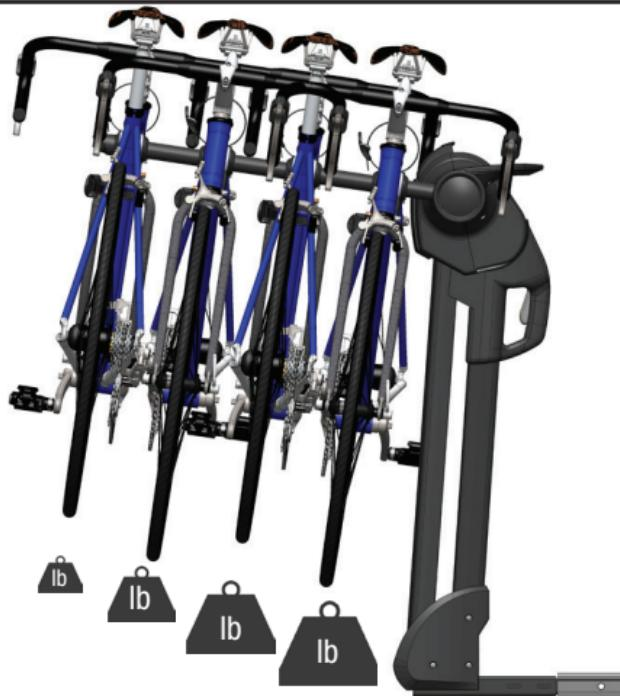
**EN** Load bikes, heaviest to lightest, with heaviest bikes closest to car. The rear of each bike should be on the same side as the anti-sway strap that hangs below the rack arm. Load bikes on the arms alternating directions.
