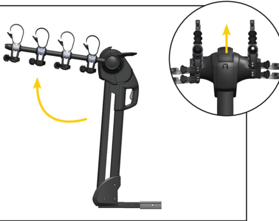
**EN** Raise rack arms up by lifting the lever at the top of the rack, then rotate arms up. You will hear an audible click when the arms are in locked position.
