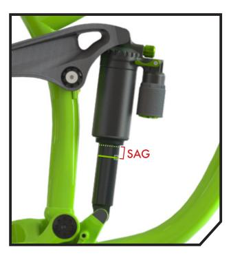
Measure the distance the O-ring has moved. Your SAG equals the distance from the O-ring to the air canister.
