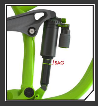
3. Measure the distance the O-ring has moved. Your SAG equals the distance from the O-ring to the air canister.
