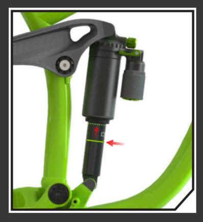
2. Move the O-ring to the top of the shaft. Mount the bike in your riding gear and in the attack position.
