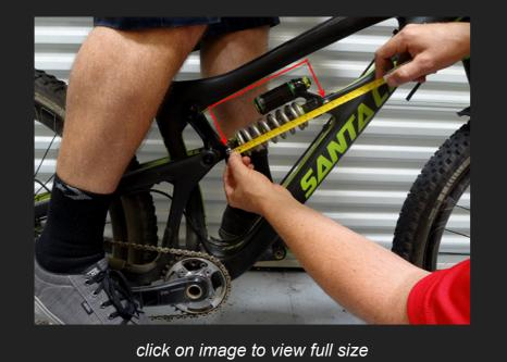
3. Now calculate the sag by taking the uncompressed eye to eye distance and subtract it from the compressed eye to eye distance.
