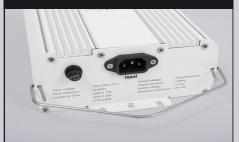
Lay the ballast flat and attach the hanging bracket into the holes on either side of the ballast casing.
